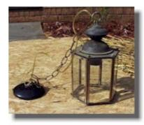
Step 4. Use a standard plastic or ceramic utility light socket as shown. Spray paint flat black. Fasten electrical cord/wire to the screws on the back of the utility light socket, and fish wire through the 3/4" holes drilled in the center of the top and bottom wood donuts of your project. Bring the wire to the square bottom cavity of the base. Fasten this light socket to the top with 2 screws.
